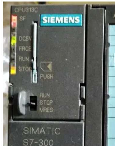
Figure 6 Siemens S7-300 Leds
